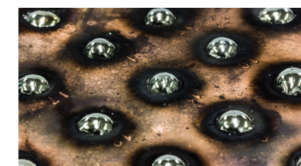
Beads of scandium metal are shown on a cast on a copper hearth plate. Scandium is one of the high-purity rare earth metals prepared for MPC customers.
