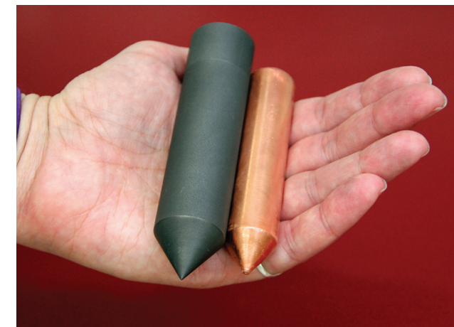
Ames Laboratory scientist Deborah Schlagel holds a graphite crucible (left) and a Bridgman-grown copper crystal (right).
