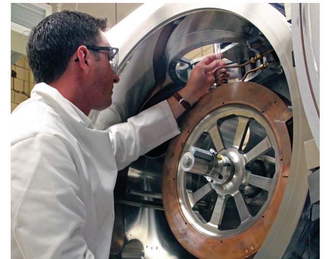
Ames Laboratory scientist Brandt Jensen loads a sample into the melt spinner. The induction coil melts the sample, which is then forced in a stream onto the spinning copper wheel.
