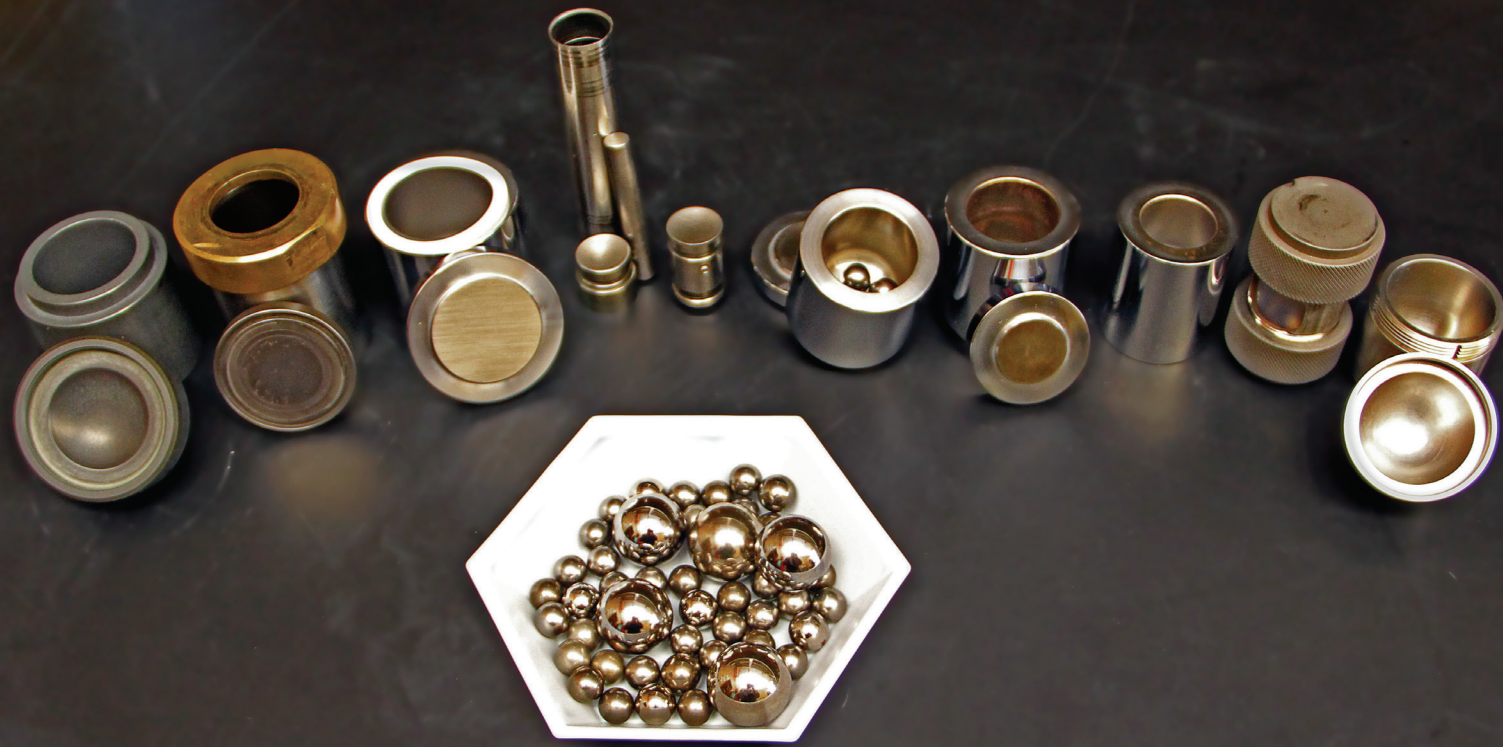
An array of ball milling canisters and stainless steel balls Vitalij Pecharsky's group uses to process materials in their solid state.
