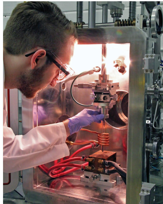
Jacob Fischer, undergraduate research assistant, loads a sample into the injection casting system. The melted material is injected into water-cooled copper molds.
