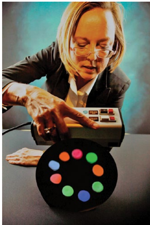
CMI researcher Nerine Cherepy, from Lawrence Livermore National Laboratory, displays phosphors developed to use far less rare-earth oxides than in current fluorescent lighting technology. CMI researchers' next goal is to develop red and green phosphors for LED lighting.
