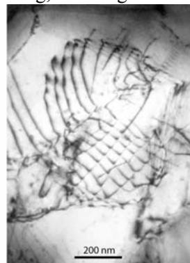
**Fig. -** (left) Comparison of the tensile test stress-strain plots of polycrystalline YAg intermetallic and commercial Al 3105 alloy; (right) TEM micrograph of dislocations in plastically deformed YAg.
