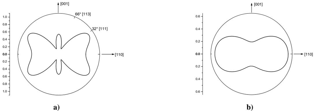
**Fig. 2** Angular variation of line tension factor of  $(1\bar{1}0)[110]$  slip dislocations, a) for NiAl, and b) for YCu.
