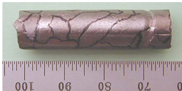
Fig. 2 Large grains of \text{Pr}_{15}\text{Ni}_{6.7}\text{Si}_{10.2} prepared by solid-state techniques from correct stoichiometries containing excess silicon.
