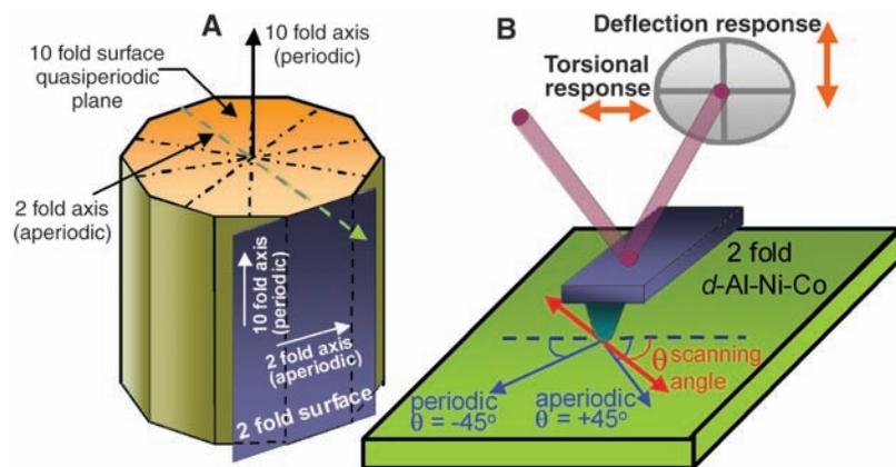
**Fig. 1.** (A) Schematic model of a decagonal Al-Ni-Co quasicrystal, showing the orientation of decagonal and twofold planes. The 2-fold plane is periodic along the 10-fold direction and aperiodic along the 2-fold direction. (B) Schematic of the cantilever and the scanning geometry during friction studies.
